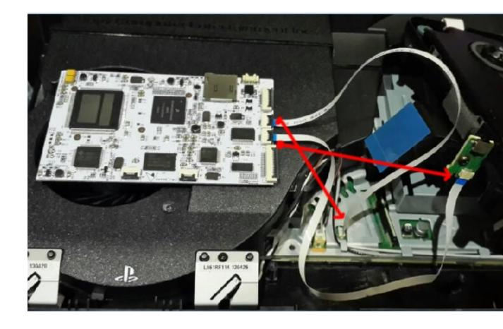
You can now connect the 7PIN FFC from E3 mainboard to E3 USB STICK
