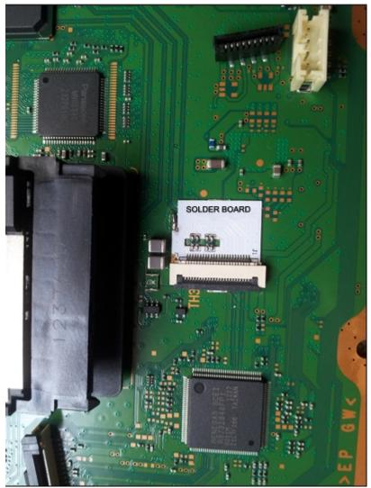
Then insert the 24 pin FFC LVDS cable (Marked as F the table above) between solder board on the ODE and 24 pin FFC LVDS connector on the solder board which you soldered to the console motherboard. 25xx/3xxx shown here:
