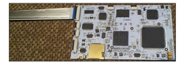
Disconnect the power cable between the console power supply and the console motherboard. Replace the cable with the correct type which has connector matching that of your console. Insert the 4 pin low profile connector to your E3 ODE PRO board connecter marked power as shown here
