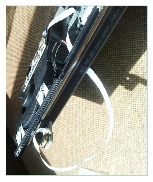
The E3 ODE PRO should be positioned inside the console as shown (CECH25XX/3XXX):
