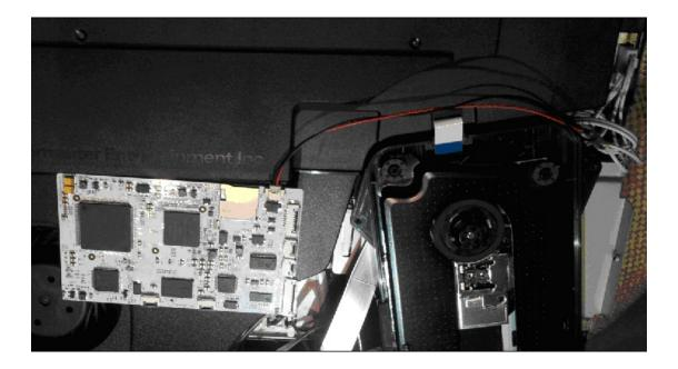
Disconnect the 6PIN eject cable between the console motherboard and the BD drive. Replace the cable with the correct type which has connector matching that of your console.
